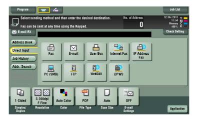
4 Directly type in the host name and file path of the destination, or tap [Reference] and specify the shared folder of the destination. Then, tap [OK].
